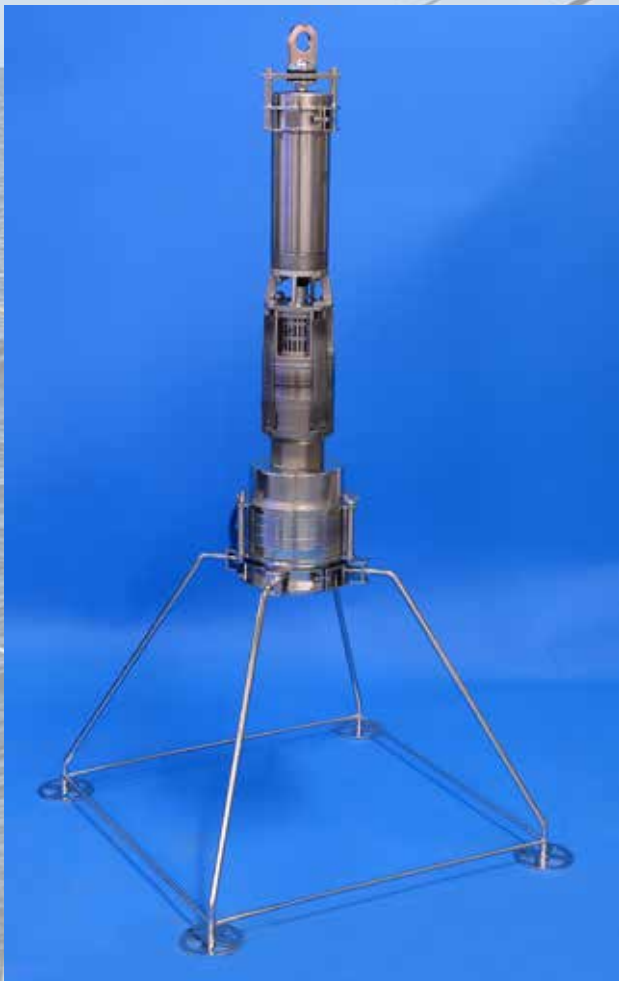
Figure 1. Microlitter sampler developed by KC Denmark in cooperation with CleanSea scientists (Image: L. Christensen).
