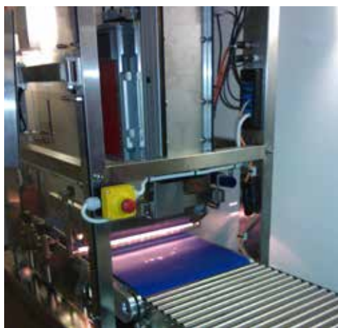
Figure 1. One of the methods being evaluated for hyperspectral image analysis. Images are collected using a linescan of the sample placed on a conveyor belt. © Schönlau
