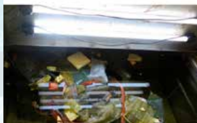
Figures 1. Marine mesocosm study of plastic degradation in the laboratory, after startup (top) and 10 months (bottom)
