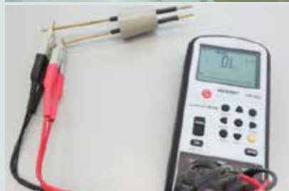
Figures 2. Test of electrical resistance measurements indicating plastic degradation
